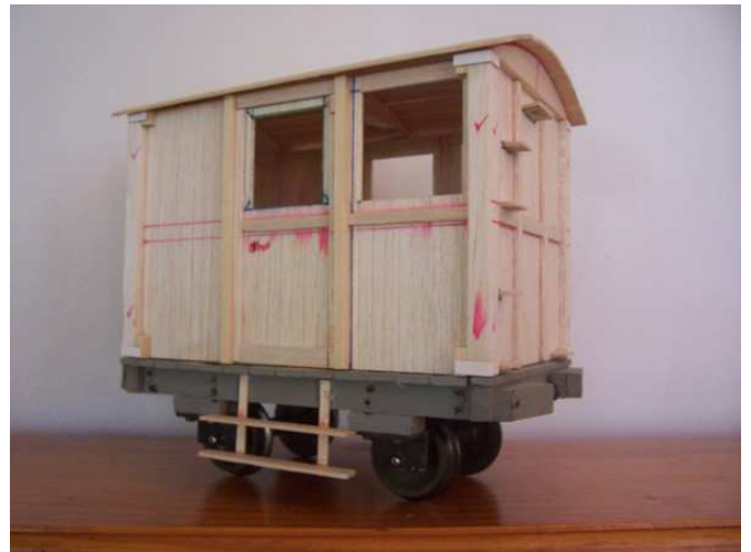
Quarry Brake Van is scratch built of wood, the wheels are Bachmann brand.
